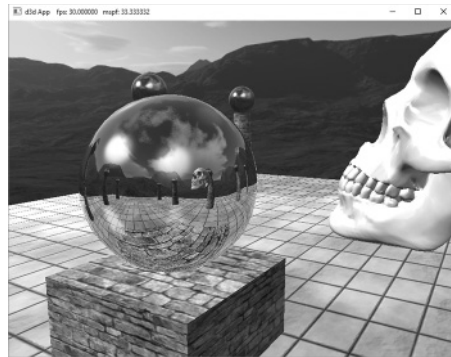
Figure 18.9. Screenshot of the “Dynamic CubeMap” demo showing off dynamic reflections. The skull orbits the center sphere, and its reflection in the sphere animates accordingly. Moreover, because we are drawing the cube maps ourselves, we can model the reflections of the local objects as well, such as the columns, spheres, and floor.
