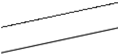
Figure 4.4. On the top we observe aliasing (the stairstep effect when trying to represent a line by a matrix of pixels) On the bottom, we see an antialiased line, which generates the final color of a pixel by sampling and using its neighboring pixels; this results in a smoother image and dilutes the stairstep effect.
