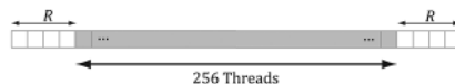
Figure 13.11. Pixels near the boundaries of the thread group will read pixels outside the thread group due to the blur radius.
