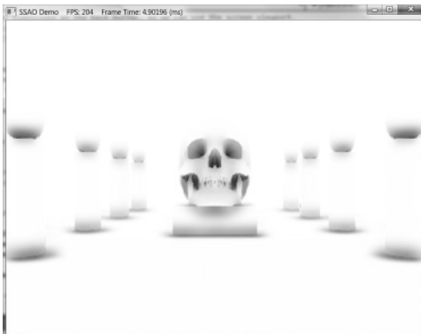
Figure 21.8. An edge preserving blur smooths out the noise. In our demo, we blur the image four times.
