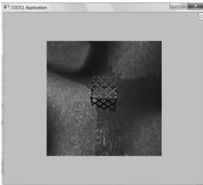
Figure 4.9. By modifying the viewport, we can draw the 3D scene into a subrectangle of the back buffer. The back buffer then gets presented to the client area of the window.
