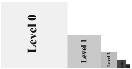
Figure 9.17. A mipmap chain manually constructed so that each level is easily distinguishable.
